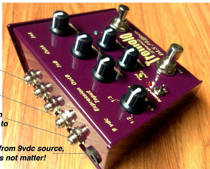
**Warmth Pot:** A first ever *Warmth* pot allows the user to dial in Vintage tube sounding tremolo to modern edgy tremolo, or any blend of the two sounds. This is achieved by biasing 2 different sounding *analog optical-couplers* via the Warmth pot.
